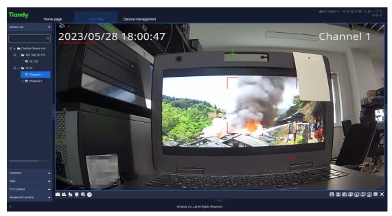
When the camera has abnormal temperature alarm, smoking alarm, fire point alarm, the software will receive the alarm and display the alarm details and pictures.
