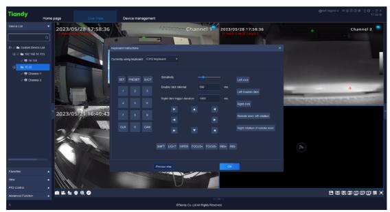
When you preview a video, you can use the keyboard to manipulate video recording, capture, and preview channel switching. You can also use the keyboard to control PTZ, set and recall preset positions, set wipers, lights, and apertures. See keyboard instructions for details.
