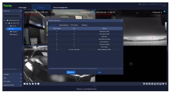
Click the debug button in the keyboard instructions to enter the keyboard debugging interface and test whether the keys of the keyboard are available normally.
